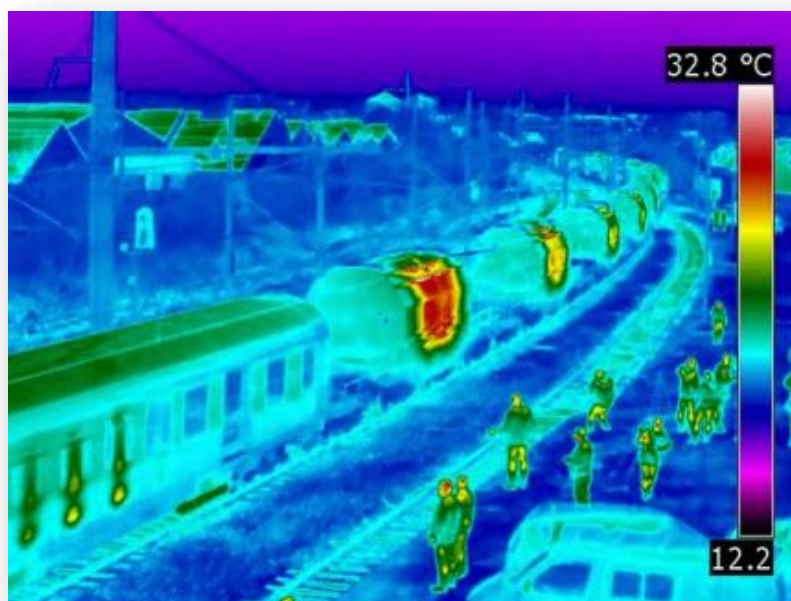
Figure 3. The sensitivity of thermal imaging is demonstrated by the hot spots seen on the outside of rail cars carrying containers of hot glassified nuclear waste being transported from France to Germany. Source: Greenpeace.
